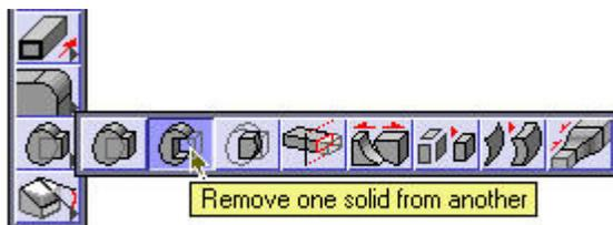
In the Message Line, it first asks for the solid to be subtracted from. That's the big one so select that one first.
