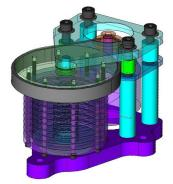
Gleeson designed this fluid-dampened servo mechanism for a camera crane with a clutch pack that applies torque without requiring a large gear train.
