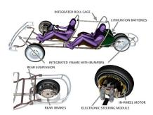
Detail of the electronic steering module with in-wheel motor.
