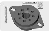
This Cobalt screen capture from THD Electronics, shows a 3D model of a phenolic octal relay socket that is essentially a copy of the old Amphenol tube socket from the'50s.
