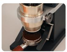
The dosing hopper (top) and the portafilter holder (bottom) are two accessories designed by John for his original espresso grinder, also designed in Xenon (centre) CAD and 3D modelling software.
